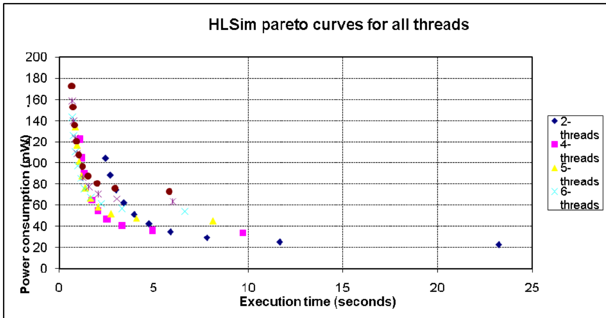
Figure 4 : Pareto graph generated by modeFRONTIER using HLSim with processor clock frequencies between 20 and 200MHz
